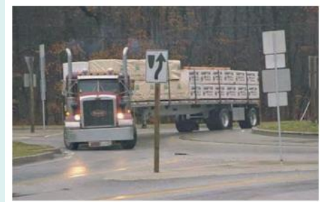
Truck using a traversable apron at a roundabout. Source: NCHRP Report 672, 2010
