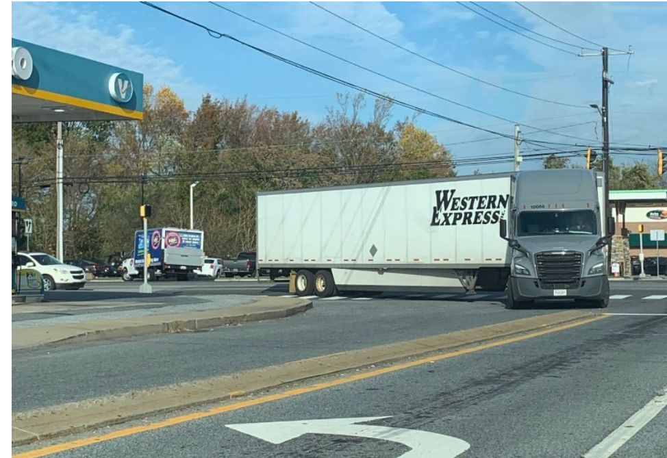
Example of tractor trailer's wide turning radius
