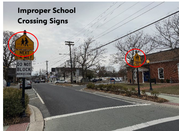
Figure 5.15: Improper School Crossing Signs SB MD 272
