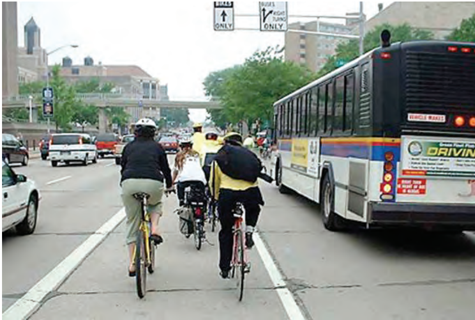
Figure 18: Left-side bike lane with right-side dedicated bus lane, University Avenue, Madison, Wisconsin 29
