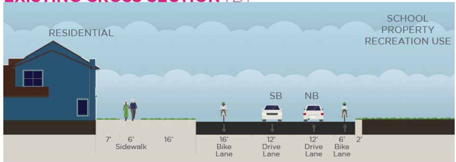
EXISTING CROSS SECTION [B]
