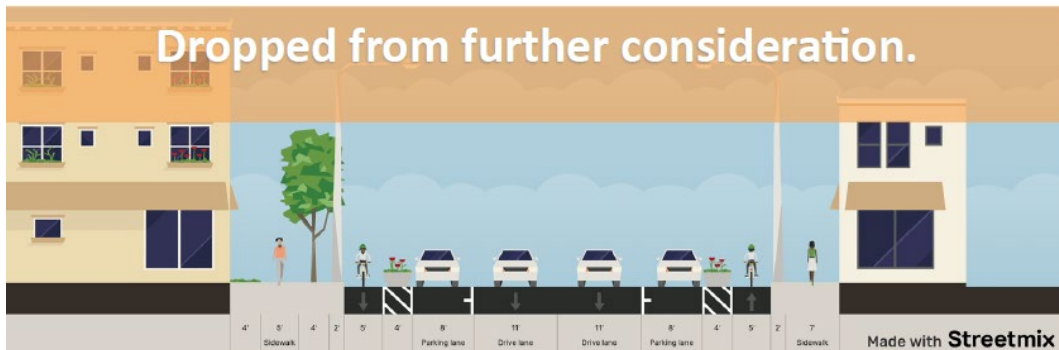
Maintain Curb Alternative 3: Parallel Parking with Two-Way Separated Bike Lanes
