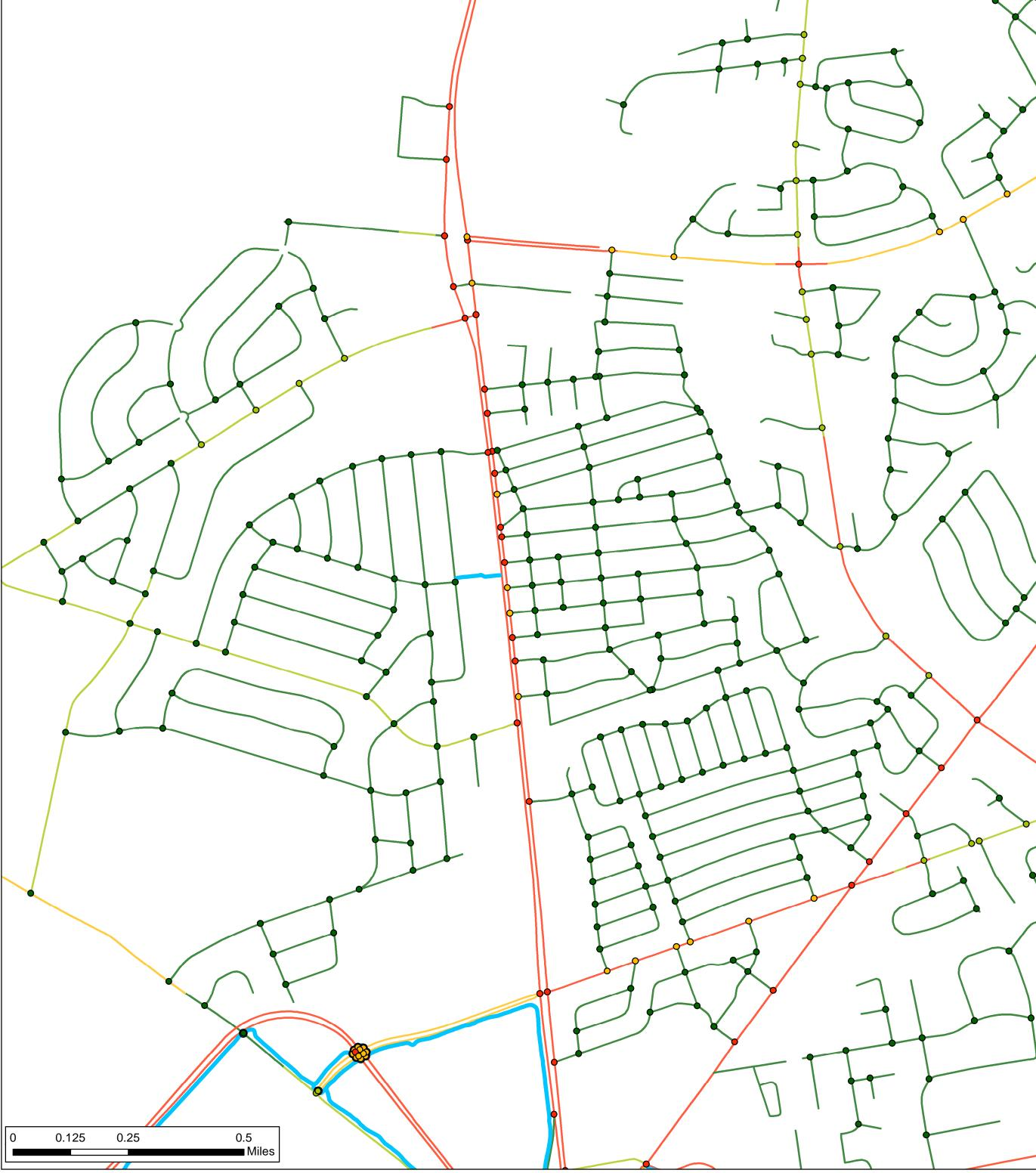
Level of Traffic Stress (LTS) is a measure being used by DelDOT to better understand how comfortable streets are for bicycle riding.
