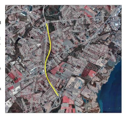
**JUSTIFICATION:** The new third lane is needed to address capacity needs along this corridor which include the need to accommodate background traffic growth as well as the new traffic that will be utilizing the new US 301 limited access highway. The concrete roadway is deteriorating and needs to be replaced.
