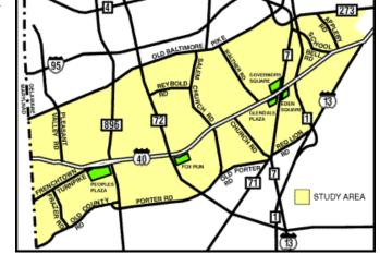
US 40 and SR 896 Grade Separated Intersection- The project consists of grade separating the intersection of US 40 and SR 896, taking SR 896 over US 40. The existing entrance to the Bristol Place development will be closed as part of the project due to its proximity to the interchange. It currently has access via George Williams Way.
